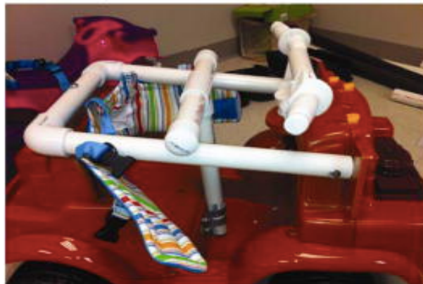
Figure 5 Roll cage on a ride-on-car with PVC pipes
